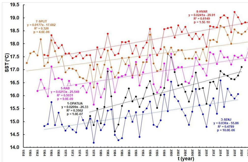
Figure 2. Time series of the mean annual SST measured at the Opatija, Senj, Rab, Split, and Hvar stations. The  $R^2$  represents the coefficient of determination, and  $p$  represents the Mann-Kendall (M-K) test values
