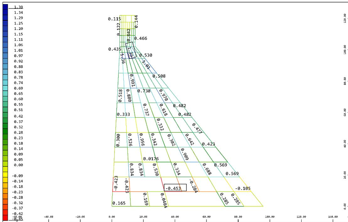
Figure 8. Display of zones of maximal tension stress,  $\sigma_{1,max}=1.40$  MPa
