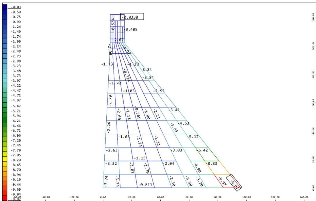
Figure 9. Display of zones of maximal compression stress,  $\sigma_{3,max}=9.97$  MPa
