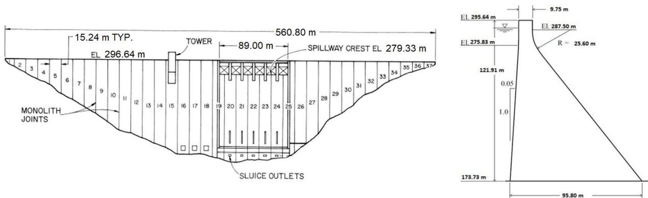
Figure 2. Downstream view of Pine Flat dam (left) and cross section geometry of monolith 16 (right)
