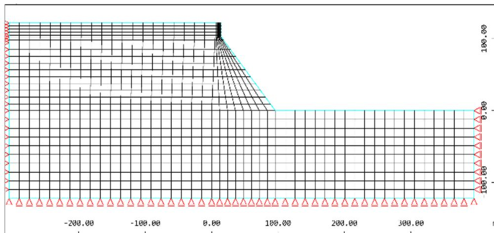
Figure 4. Display of coarse finite element mesh (N=816), applied for the Case Study
