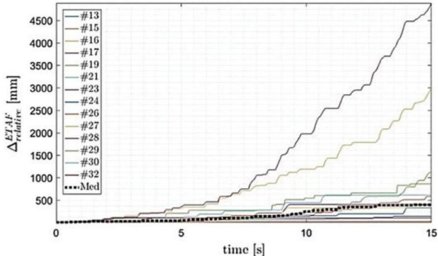
Figure 6. Displacement evolution of the relative crest displacement (node C) under ETAF excitation record [14]
