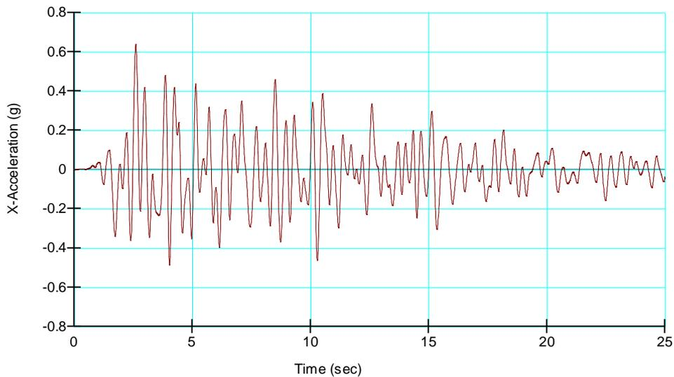
Fig. 10: Absolute acceleration  $a [g] \div t [s]$  in a horizontal direction, dam 2-2, elevation 654.0 m ASL, for the initial water level in the lagoon on 652.0 m ASL
