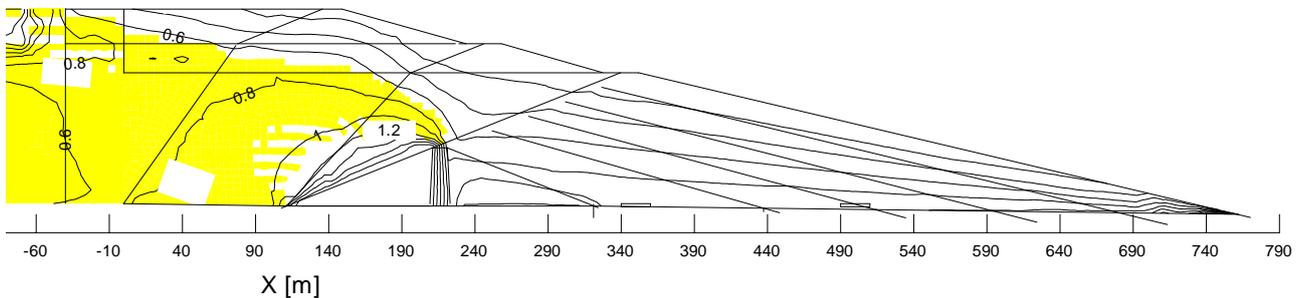
Fig. 7.2: Distribution of the parameter  $q/p$  [-] with the liquefaction zone, for the initial stress state and steady seepage for water level in the lagoon on 649.0 m ASL, with upstream seepage boundary at 700 m from the dam 2-2
