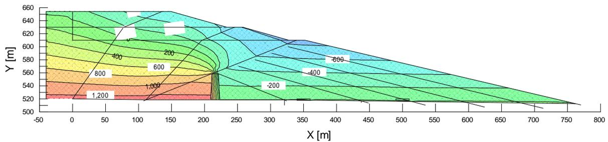
Fig. 3.1: Pore pressure distribution in kPa, for steady seepage in the tailings dam, at upper water elevation at 649.0 m ASL, with upstream seepage boundary at 150 m from the dam 2-2,  $P_{w,max} = 1,279.8$  kPa
