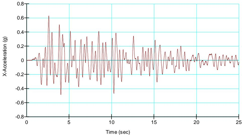
Fig. 9: Absolute acceleration  $a [g] \div t [s]$  in a horizontal direction, dam 2-2, elevation 654.0 m ASL, for the initial water level in the lagoon on 649.0 m ASL
