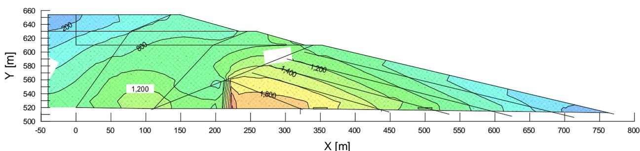
Fig. 6: Maximal effective stresses distribution, in kPa, for steady seepage in the tailings dam, at upper water elevation at 652.0 m ASL,  $S1'_{max} = 2,250.8$  kPa
