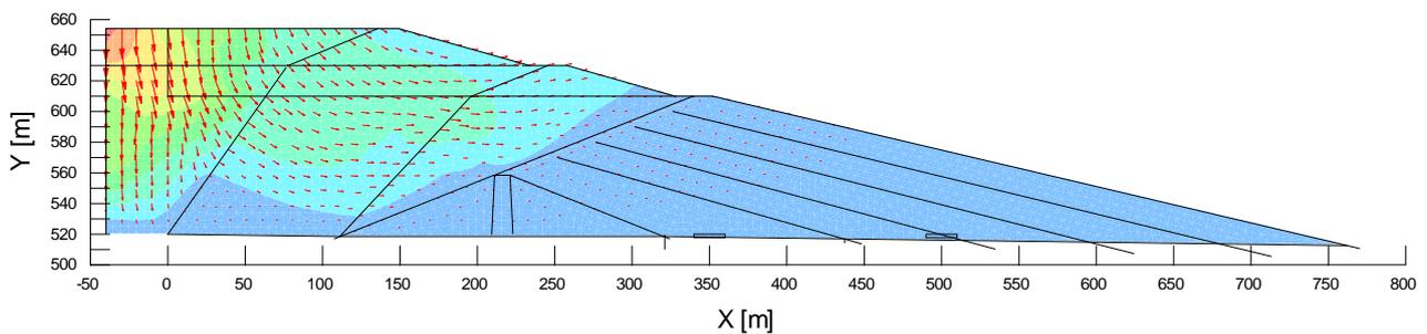
Fig. 14: The direction and intensity of the resulting displacements  $XY$ , after the earthquake, for the initial steady seepage for water level in the lagoon on 649.0 m ASL
