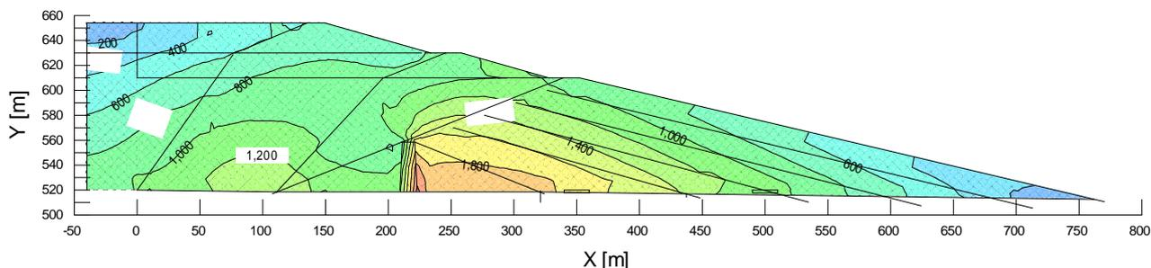
Fig. 5: Maximal effective stresses distribution, in kPa, for steady seepage in the tailings dam, at upper water elevation at 649.0 m ASL,  $S1'_{max} = 2,256.0$  kPa
