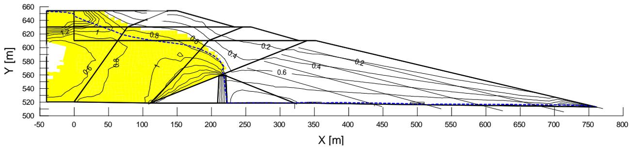
Fig. 13: Distribution of the parameter  $q / p' [-]$  with the liquefaction zone after the strong earthquake, for the initial steady seepage for water level in the lagoon on 652.0 m ASL
