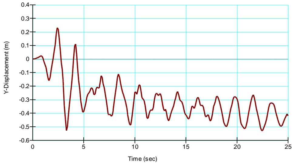
Fig. 11.1: Permanent vertical displacements obtained by the dynamic deformation method,  $Y [m] \div t [s]$ , in the upstream crest edge of the dam 2-2, at level 654.0 m ASL, for the initial water level in the lagoon on 649.0 m ASL, with upstream seepage boundary at 150 m from the dam 2-2
