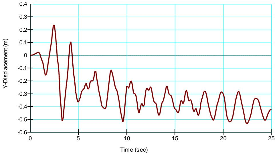
Fig. 12: Permanent vertical displacements obtained by the dynamic deformation method,  $Y [m] \div t [s]$ , in the upstream crest edge of the dam 2-2, at level 654.0 m ASL, for the initial water level in the lagoon on 652.0 m ASL
