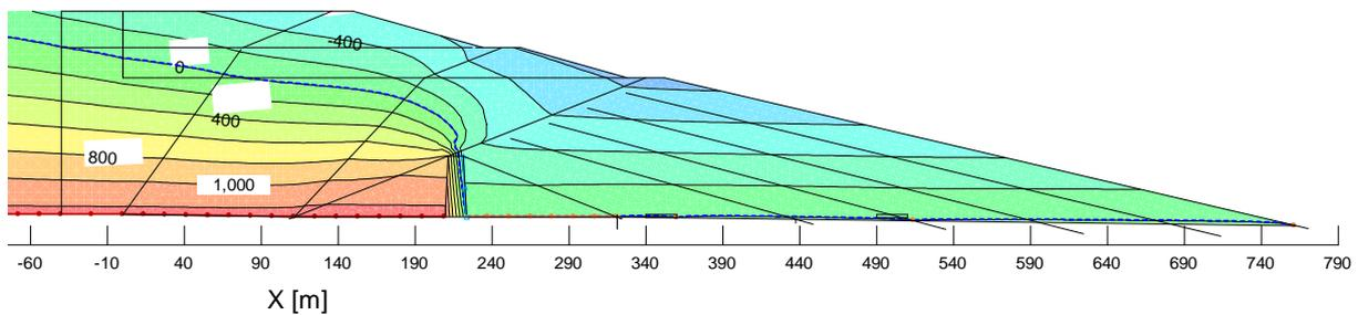
Fig. 3.2: Pore pressure distribution in kPa, for steady seepage in the tailings dam, at upper water elevation at 649.0 m ASL, with upstream seepage boundary at 700 m from the dam 2-2,  $P_{w,max} = 1,279.8$  kPa
