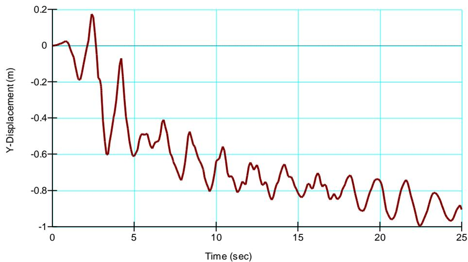
Fig. 11.2: Permanent vertical displacements obtained by the dynamic deformation method,  $Y [m] \div t [s]$ , in the upstream crest edge of the dam 2-2, at level 654.0 m ASL, for the initial water level in the lagoon on 649.0 m ASL, with upstream seepage boundary at 700 m from the dam 2-2
