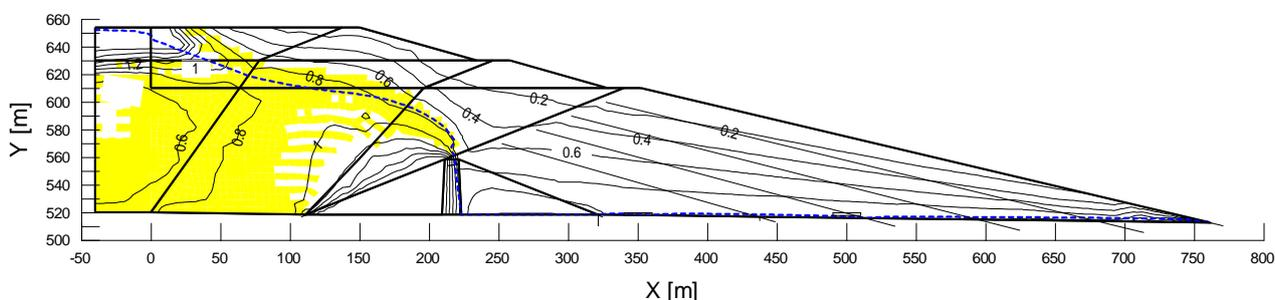
Fig. 8: Distribution of the parameter  $q/p$  [-] with the liquefaction zone, for the initial stress state and steady seepage for water level in the lagoon on 652.0 m ASL
