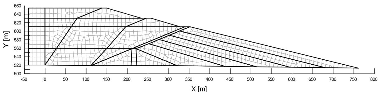
Figure 2: Discretization of the mediums for static analysis by FEM (Nodes=810, Elements=766), with upstream seepage boundary at 150 m from the dam 2-2
