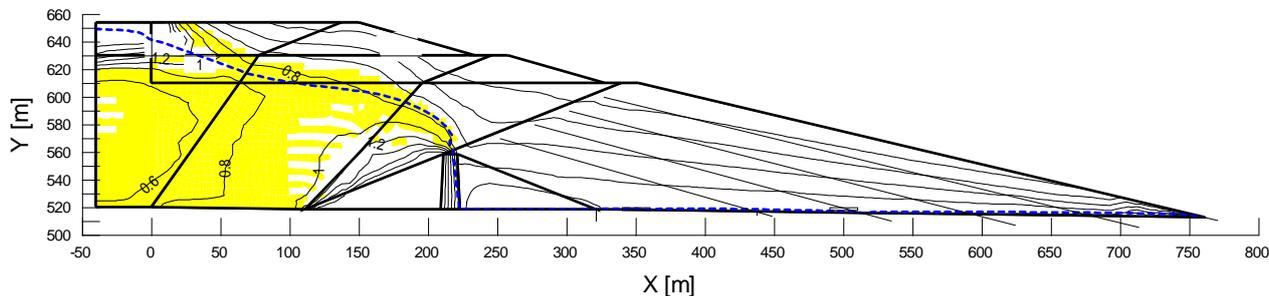
Fig. 7.1: Distribution of the parameter  $q/p$  [-] with the liquefaction zone, for the initial stress state and steady seepage for water level in the lagoon on 649.0 m ASL, with upstream seepage boundary at 150 m from the dam 2-2
