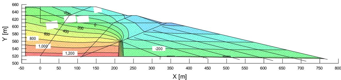
Fig. 4: Pore pressure distribution in kPa, for steady seepage in the tailings dam, at upper water elevation at 652.0 m ASL,  $P_{w,max} = 1,309.2$  kPa
