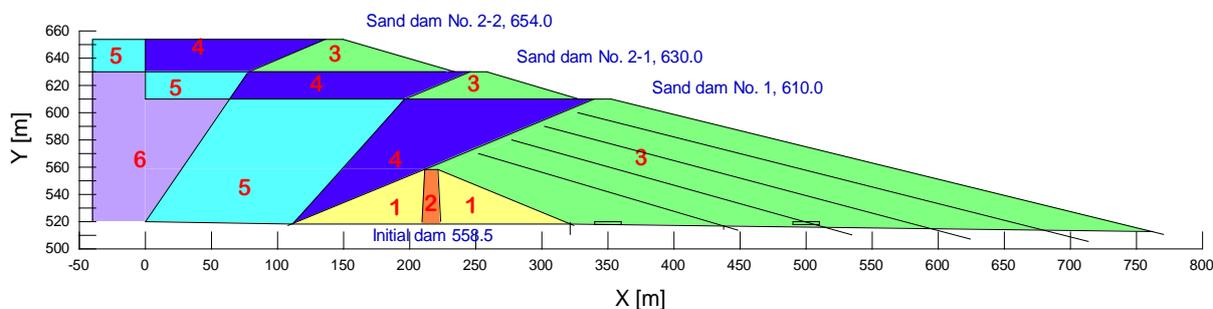
Fig. 1: Segments by six different materials. 1 – gravel in initial dam body, 2 – clay in initial dam core, 3 – sand in tailings dam, 4 – sand silt in beach, 5 – sand silt between the beach and lagoon and 6 – silt in waste lagoon
