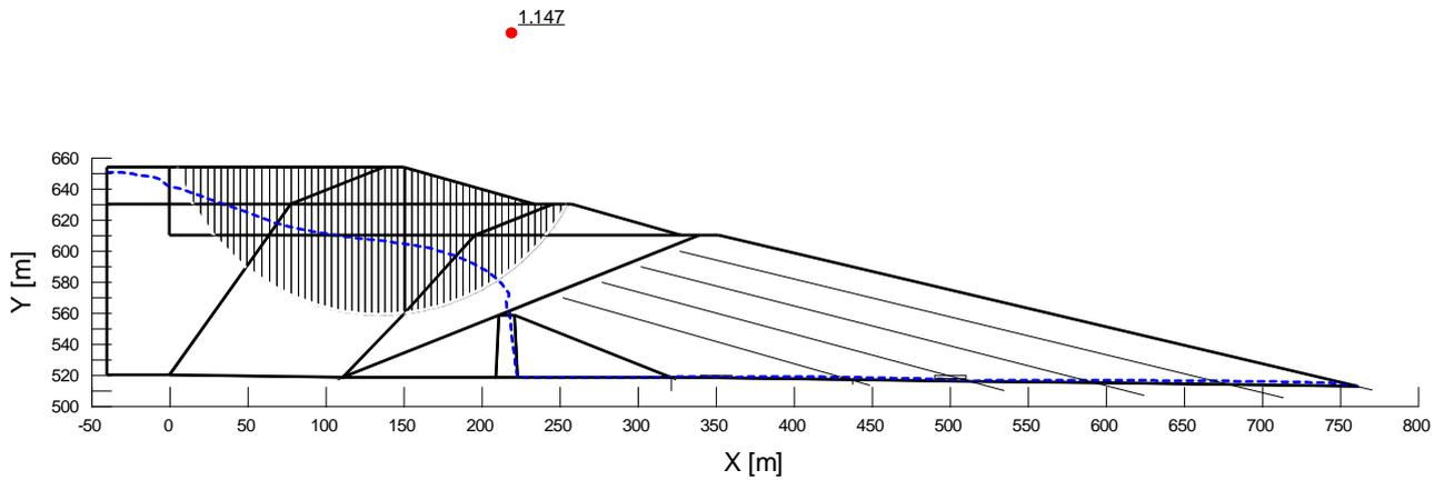
Fig. 15.1: Critical sliding surface, in the post-earthquake phase, with a stability factor  $F = 1.147$ , for the initial steady seepage for water level in the lagoon on 649.0 m ASL, with upstream seepage boundary at 150 m from the dam 2-2
