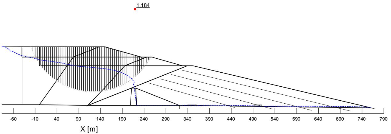
Fig. 15.2: Critical sliding surface, in the post-earthquake phase, with a stability factor  $F = 1.184$ , for the initial steady seepage for water level in the lagoon on 649.0 m ASL, with upstream seepage boundary at 700 m from the dam 2-2
