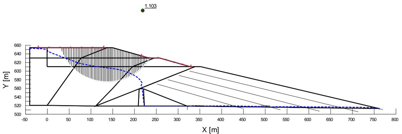
Fig. 16: Critical sliding surface, in the post-earthquake phase, with a stability factor  $F = 1.103$ , for the initial steady seepage for water level in the lagoon on 652.0 m ASL
